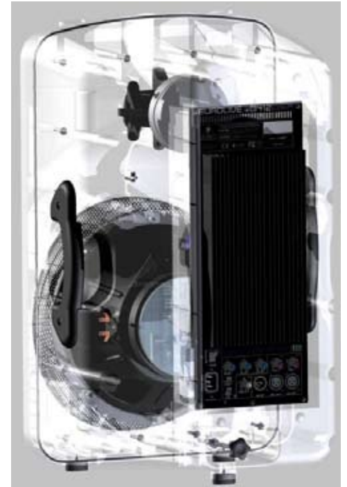
Image courtesy of Behringer. Analysing and optimizing the volume of a speaker enclosure in Autodesk Inventor
